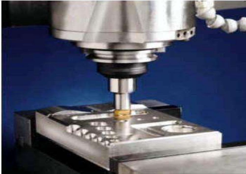
End milling operation used to cut a pocket in an aluminum work part.
