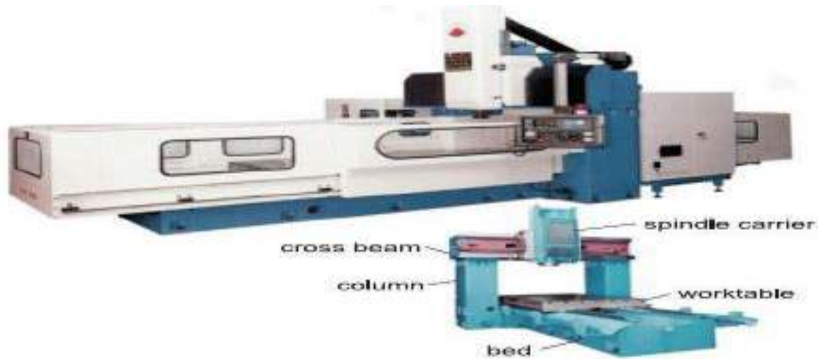
Portal planer mill for heavy machining of large workparts.
